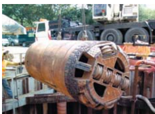
Bit replacement inside of machine
