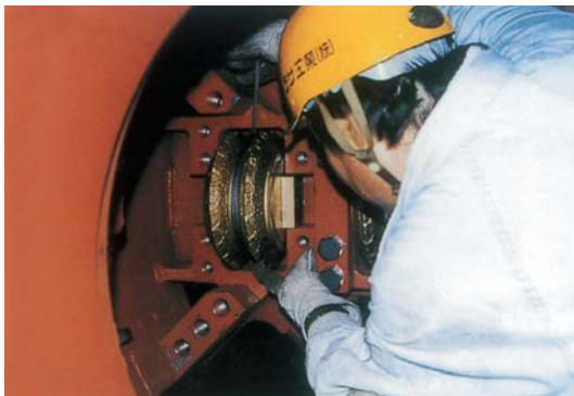
Bit replacement inside of machine
